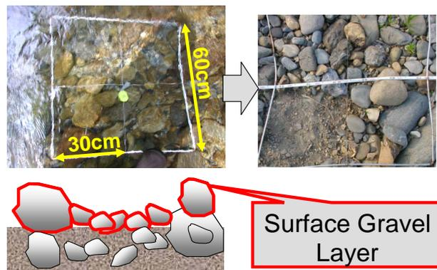
**Fig.3** The quadrat we used and the schematic image of surface gravel layer
