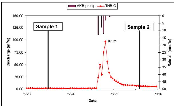
**Fig.2** Hydrograph near the AFB site. Pre- and post-flood observation times are also shown.
