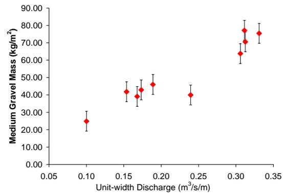
**Fig.10** Relationship between averaged unit-width discharge and averaged medium-sized gravel mass in ten riffles around the target sites in this study
