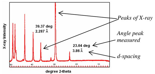
**Fig.6** X-ray diffraction pattern of sediment sample
