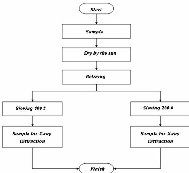
**Fig.4** Processing X-ray powder diffraction for mineralogy decomposition
