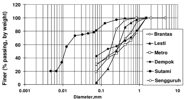
**Fig. 9** Grain size distribution of sediment from Brantas and Lesti sub-basins and deposited in Sengguruh reservoir
