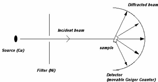
**Fig.5** Schematic of an X-ray powder diffractometer
