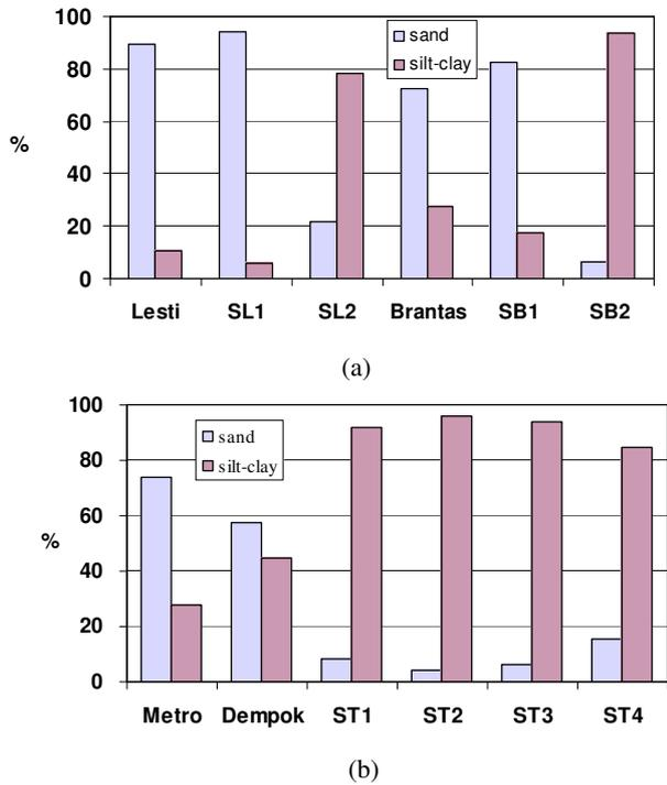
**Fig.7** Percentages of sand and silt-clay mineral between deposited and sources material in Sengguruh (a) and Sutami (b) reservoirs
