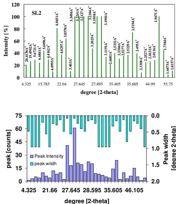
**Fig.11** Example analysis of XRD results for Sengguruh reservoir (SL2)
