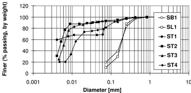
**Fig.8** Comparison of grain size distribution of deposited material in Sengguruh and Sutami reservoirs
