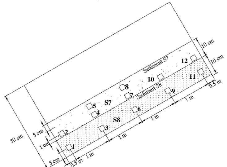
**Fig. 7** Arrangement of WCRs (1-12) in experiment II (upper layer S7 and lower layer S8)
