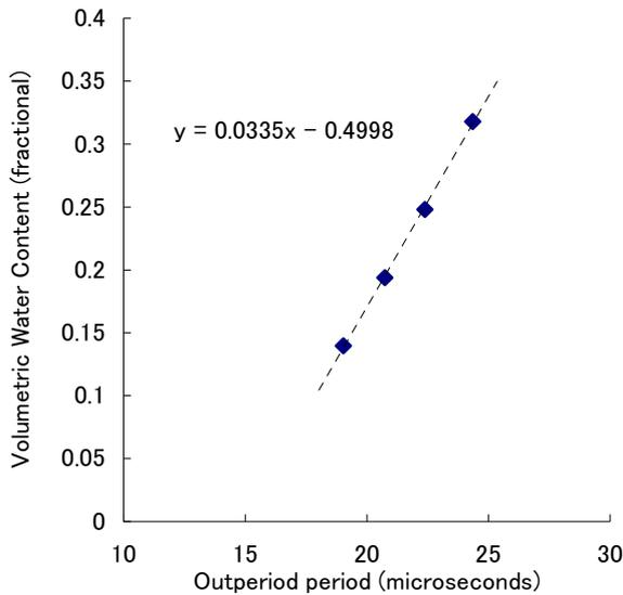
**Fig. 2** Typical quadratic calibration curve for WCR-1 and S8
