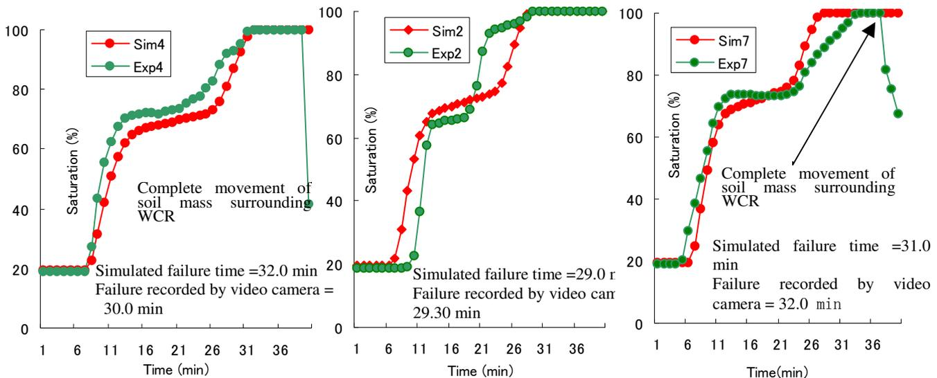
**Fig.8** Experimental and simulated results of the water content profile and landslide time (WCR-4, 2and 7)
