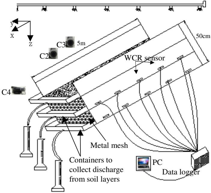
**Fig. 1** Overview of experimental setup, instrumentation and data logging system. C1,C2,C3 and C4 are video cameras
