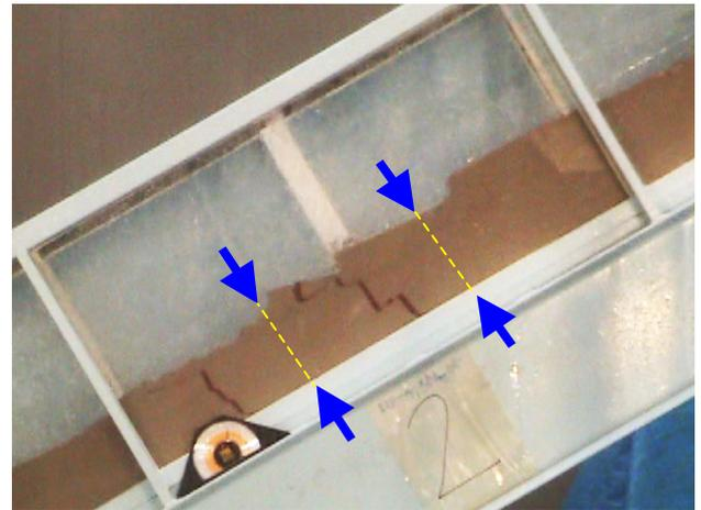
**Fig. 6** Slide of whole 20cm depth in first experiment; yellow lines (between blue arrows) show original positions of red strips (initially 1.33m and 1.66m from downstream end)
