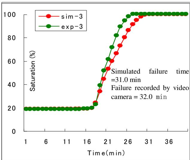
**Fig.5** Numerical Simulation and experimental result of moisture Saturation (%) on single layered soil
