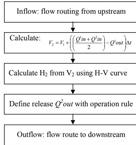
Fig.2 Flowchart of reservoir operation module
