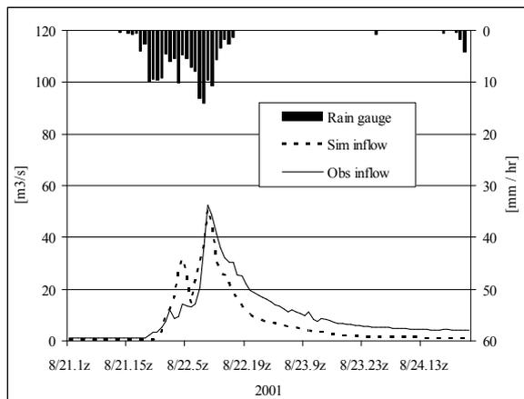
**Fig.3** Inflow to Shimagawa dam using rain gauge
