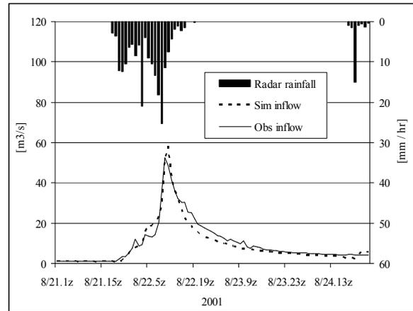
**Fig.4** Inflow to Shimagawa dam using radar rainfall
