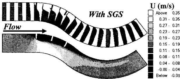
Fig.6 Time averaged-velocities (50 th -100 th sec interval) in the case of three dikes existing in the model.
