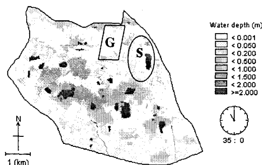
Fig.15 The inundation water depth after 35 hr
