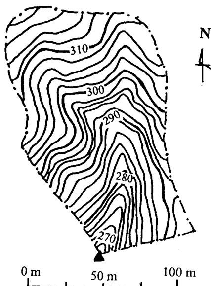
Fig. 4 Topographic map of Shomasama Subcatchment (Elevation is in meter and contour interval is 2 m)
