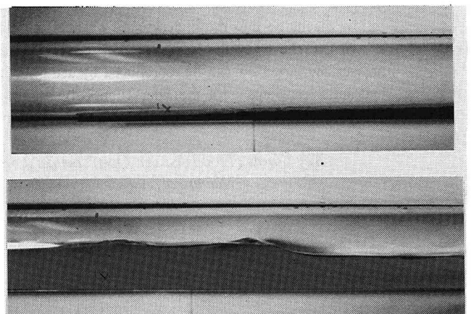
Photo 1 Invasion process of water front and the propagation of hydraulic bore
