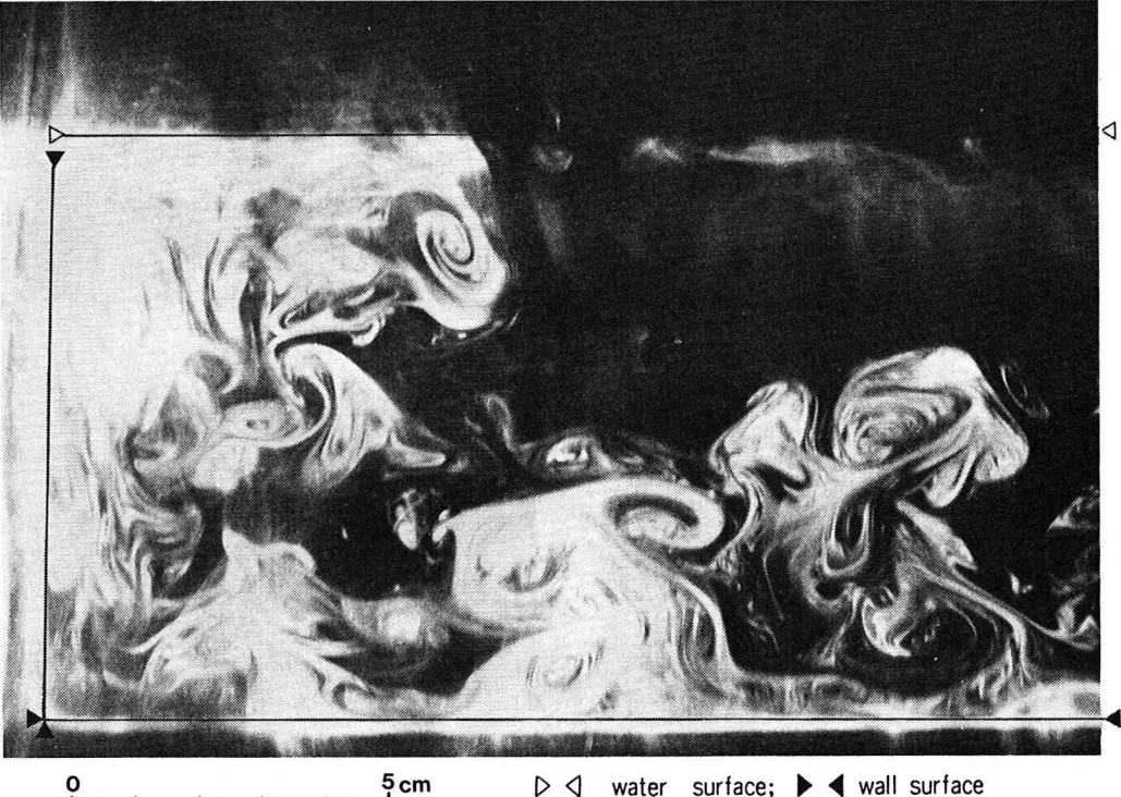
Fig. 6. An enlarged photograph of the coherent structure of the turbulent corner flow.
