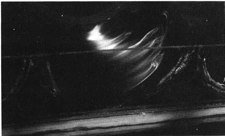
Photo.2 The Görtler vortices appeared on the trough. Dune model; Cusp head 1, R=978 . The towed direction of the model is from left to right. (after Nakagawa 6 ).
