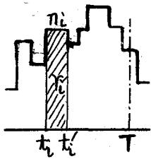
$$q_i(t) = \{\alpha(t-t_i)-1+e^{-\alpha(t-t_i)}\} r_i A / m \alpha \quad t_i \leq t \leq t_i + n_i \quad (1)$$
