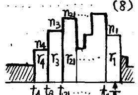
$$\left. \begin{aligned} q_4(t) &= (e^{\alpha n_4} - 1)(e^{\alpha m} - 1) e^{-\alpha(t-t_4)} r_4 A / m \alpha \\ q_3(t) &= \{\alpha(m+n_3+t_3-t)+1-e^{-\alpha(t-t_3)}(e^{\alpha m}+e^{\alpha n_3}-1)\} r_3 A / m \alpha \\ q_2(t) &= \{\alpha n_2 - (e^{\alpha n_2} - 1) e^{-\alpha(t-t_2)}\} r_2 A / m \alpha \\ q_1(t) &= \{\alpha(t-t_1)-1+e^{-\alpha(t-t_1)}\} r_1 A / m \alpha \end{aligned} \right\} \quad (9)$$
