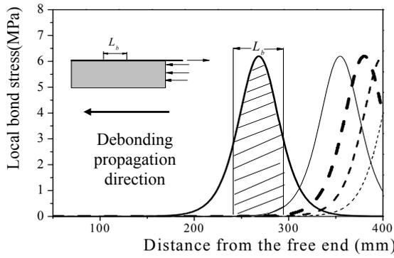
Fig. 4 Typical shear bond stress distribution in FRP/concrete joints under a simple shear test
