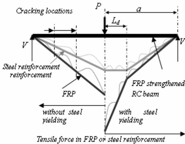
Fig. 1 Difference in tensile stress profile in FRP before and after steel yields
