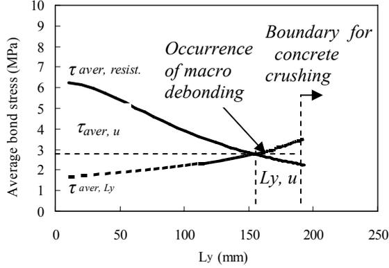
**Fig. 3** Typical relationship between the average bond stress in FRP/concrete interface within the yielding zone and the steel yielding length
