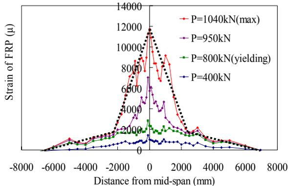
Fig.2 Strain profiles of FRP in a large-span RC deck strengthened with FRP(Dai et al. 2005a)
