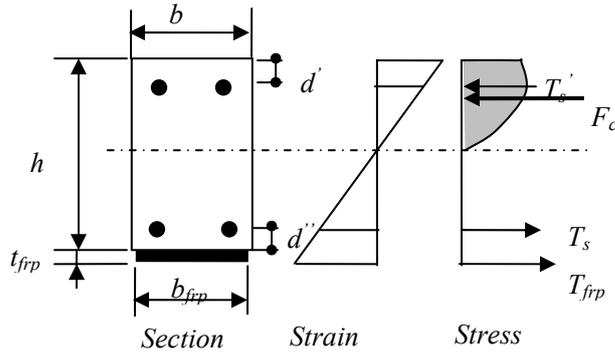
Fig. 5 Stress and strain profiles of FRP strengthened cross section
