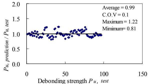
Fig.8 Comparison between predicted and experimental load-carrying capacity
