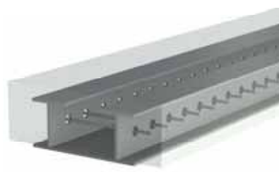
(c) Embedded type : Perforated rib
