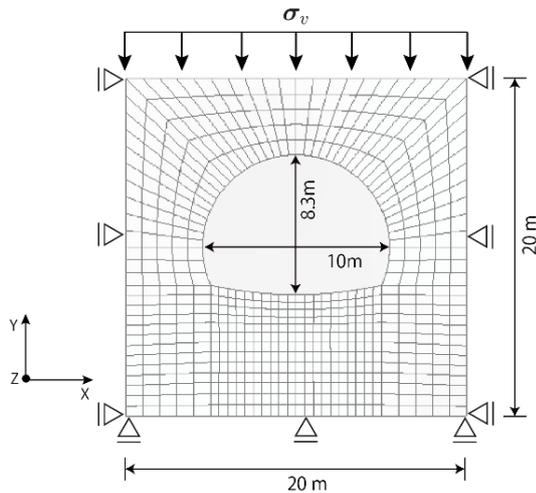
**Fig.1** Model for initial stress analysis
