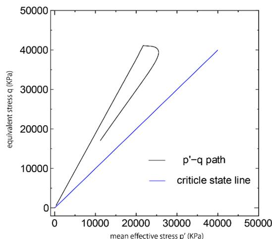
Fig.6 Stress path of swelling process
