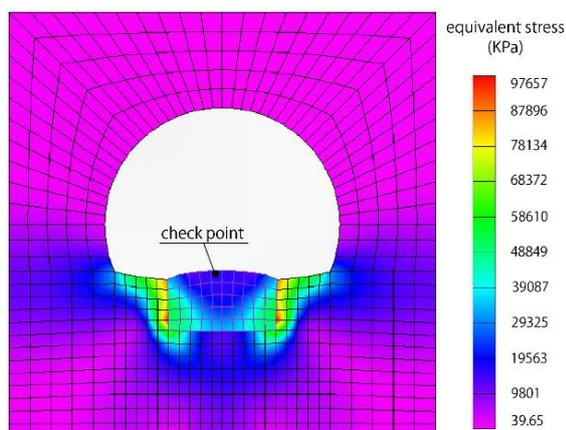
Fig.5 Equivalent stress distribution
