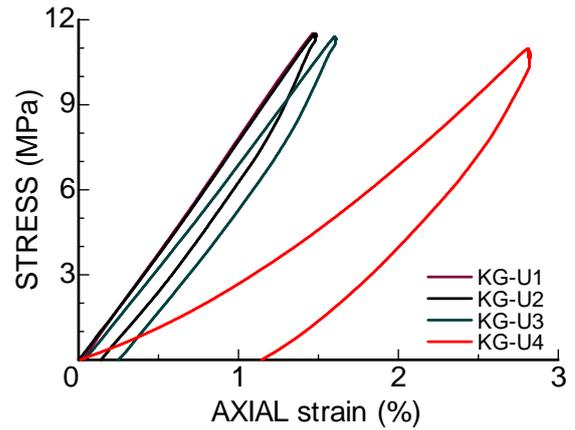
Figure 11. Strain-stress responses of Kaore granite samples
