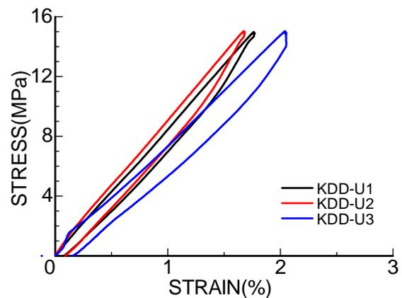
Figure 14. Strain-stress responses of Daitojima dolomite samples subjected to compression
