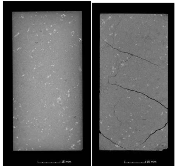
Figure 7. X-Ray images of KG-U4 sample before and after thermal shock.
