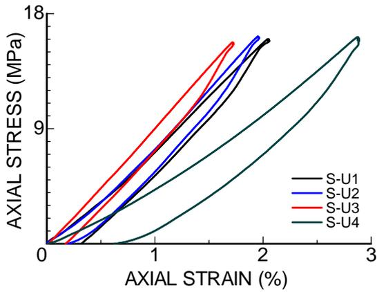
Figure 12. Strain-stress responses of Shakudani tuff samples subjected to compression.
