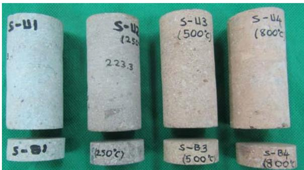
Figure 5. Views of Shakudani tuff samples after thermal shocks except S-U1 sample.
