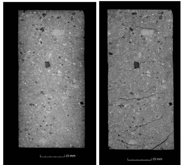
Figure 8. X-Ray images of S-U4 sample before and after thermal shock
