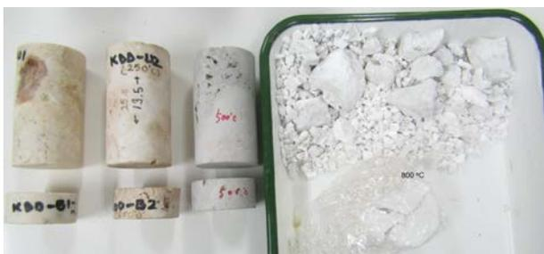
Figure 6. Views of Daitojima dolomite samples after thermal shocks except KDD-U1 sample.
