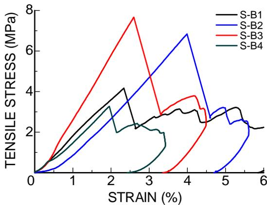
Figure 13. Strain-stress responses of Shakudani tuff samples in Brazilian tests.
