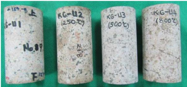
Figure 4. Views of Kaore granite samples after thermal shocks except KG-U1 sample.
