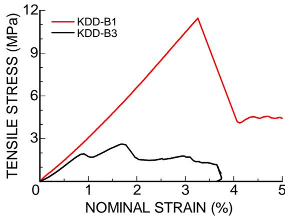
Figure 15. Strain-stress responses of Daitojima dolomite samples in Brazilian tests.
