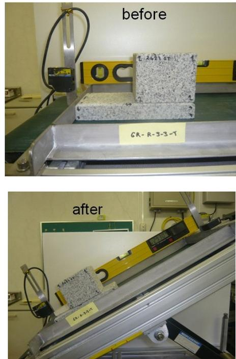
Figure 8. Views of tilting experiment on rough discontinuity plane of granite
