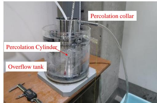
**Fig. 3** Apparatus of permeability test in Kyoto University
