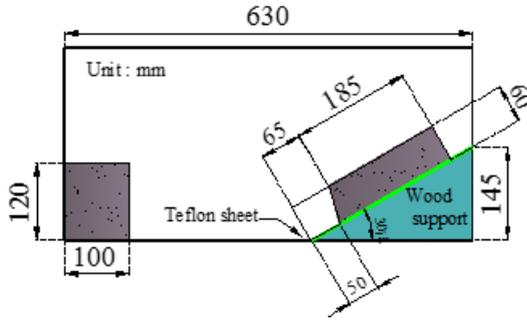
Fig. 5 The sizes of the rectangular block sand and the trapezoidal slope
