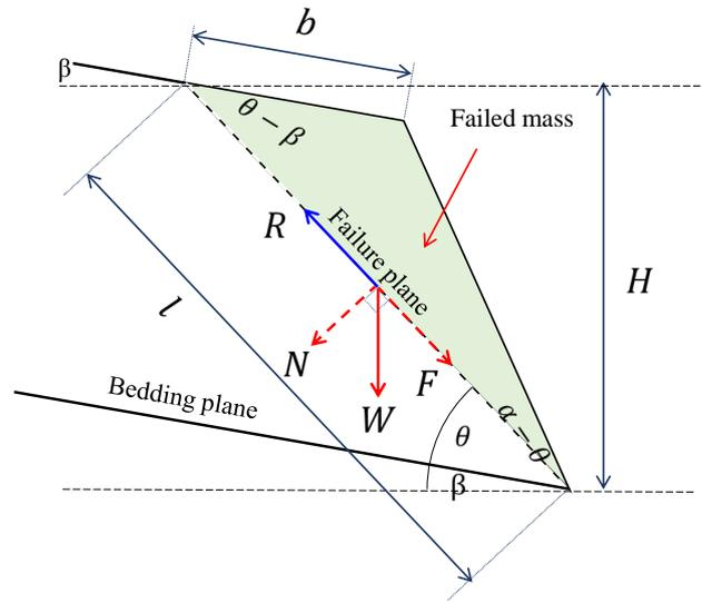
**Fig. 9** Force diagram of a trapezoidal slope
