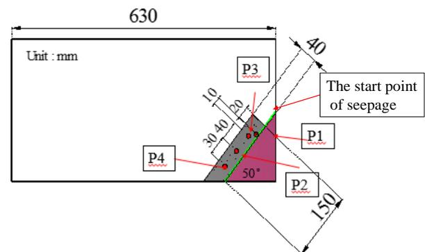
**Fig.11** Schematic diagram of the experimental slope model and the pressure gauges locations
