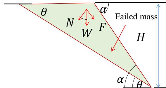
Fig. 7 Force diagram of a sand block
