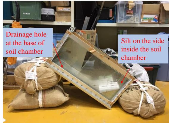
**Fig. 10** Soil chamber and rotation for the compaction process
