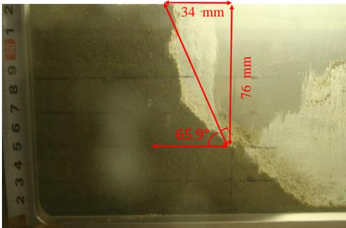
Fig. 6 Partial failure of the rectangular block
