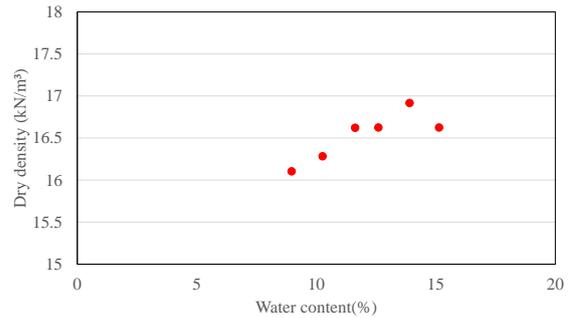
**Fig. 2** Compaction curve of Hiroshima sand.
