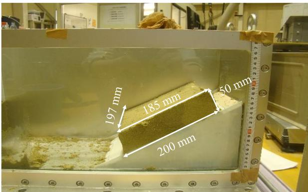
(a) A trapezoidal slope before test
