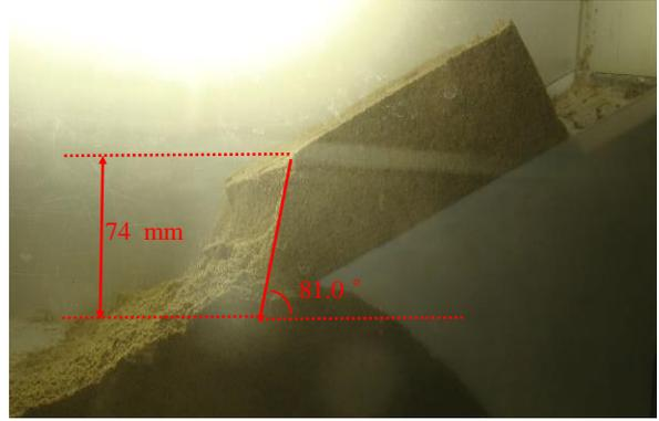
(b) A trapezoidal slope after test
