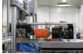
Fig. 3 MTS direct shear test machine
