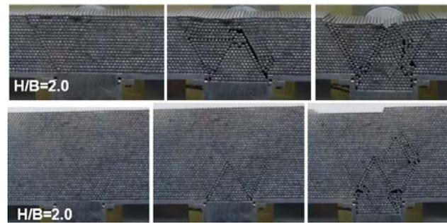
Figure 7. Views of models before and after excavation with an overburden ratio (H/B) of 1.0 and 2.0 using aluminium bars as model ground.
