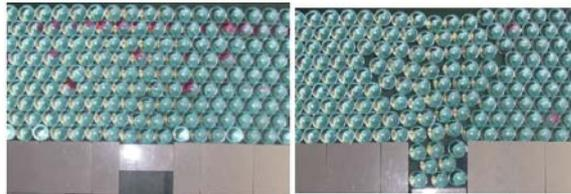
Figure 6. Views of models before and after excavation with an overburden ratio (H/B) of 2.0 using glass-beads as model ground.
