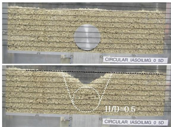
Figure 2. Views of models before and after excavation with an overburden ratio (H/D) of 0.5.
