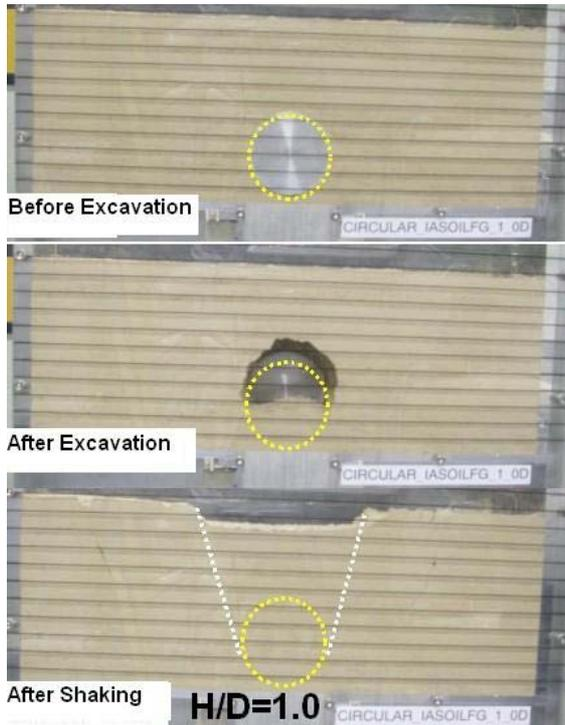
Figure 1. Views of models before and after excavation and after shaking.
