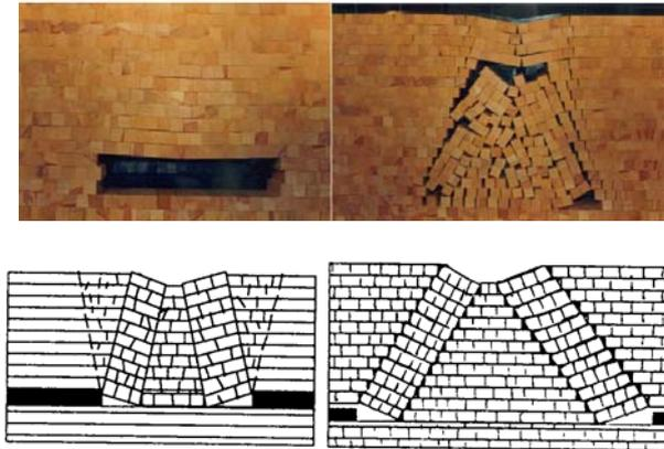
Figure 5. Views and illustrations of a rectangular underground opening in layered and jointed rock mass model.
