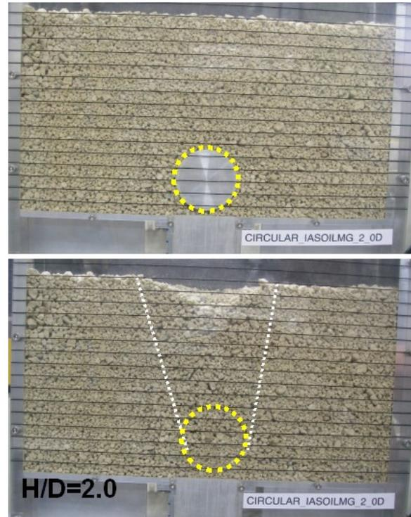
Figure 3. Views of models before and after excavation with an overburden ratio (H/D) of 2.0
