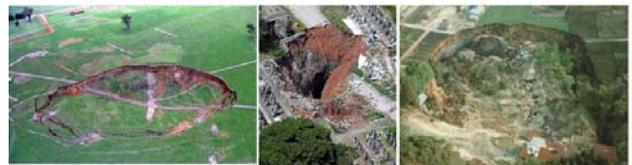
Figure 11. Surface depressions due to collapses of man-made underground cavities.
