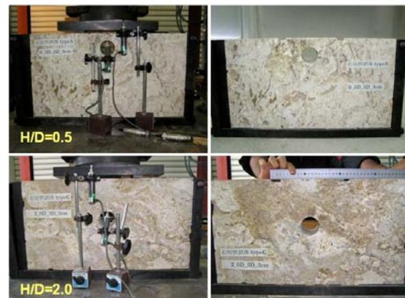
Figure 8. Footing tests on Ryukyu limestone blocks having circular cavities.
