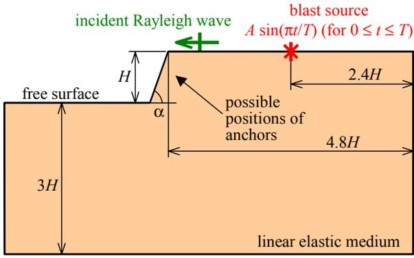
Fig.4 The numerical model for wave interaction with an arbitrarily inclined slope with a convex/concave shape.
