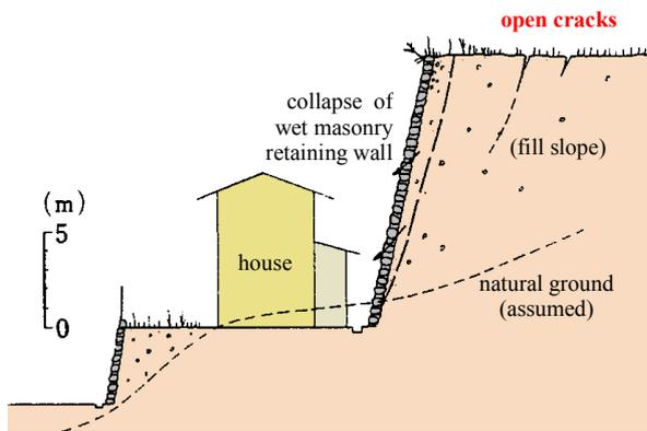
Fig.1 Typical failure of a fill slope found in Sendai, Japan, on the occasion of the 1978 Miyagi-ken-oki earthquake (modified after OYO<sup>2</sup>).
