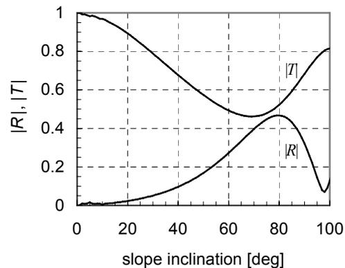
Fig.3 The effect of the slope inclination  $\alpha$  on the reflection and transmission coefficients,  $|R|$  and  $|T|$ , respectively, for Poisson's ratio 0.25.
