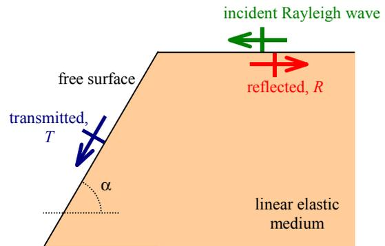
Fig.2 The slope model employed in the analysis.
