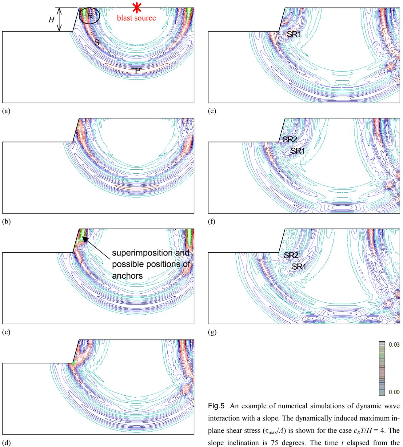
Fig.5 An example of numerical simulations of dynamic wave interaction with a slope. The dynamically induced maximum in-plane shear stress ( $\tau_{\max}/A$ ) is shown for the case  $c_R T/H = 4$ . The slope inclination is 75 degrees. The time  $t$  elapsed from the ignition of explosives at the blast source is normalized as  $c_R t/H =$  (a) 15.9; (b) 17.5; (c) 19.1; (d) 20.7; (e) 22.3; (f) 23.9; and (g) 25.5.
