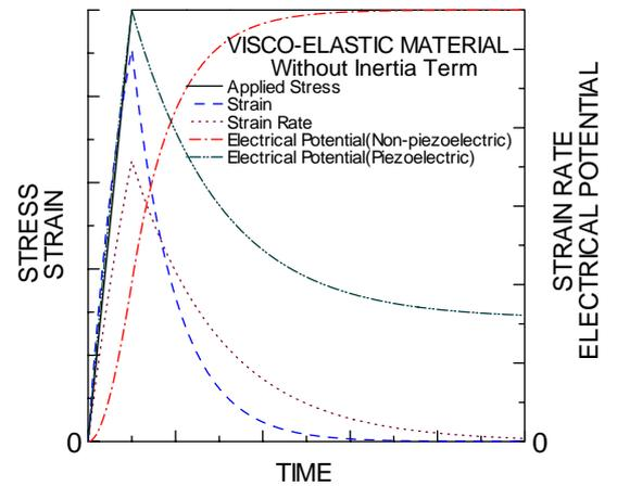
Figure 11: Computed responses of various parameters during a uniaxial loading without consideration of inertia
