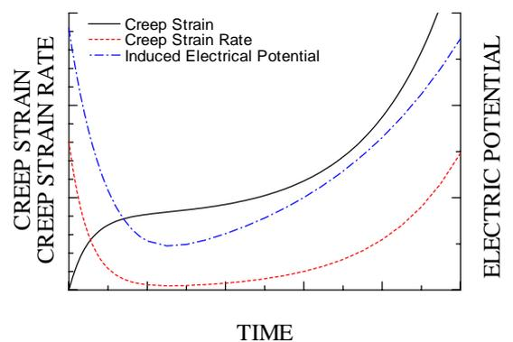
Figure 12: Computed responses of various parameters during creep failure
