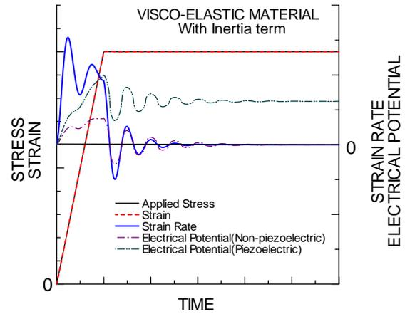
Figure 10: Computed responses of various parameters during a uniaxial loading with consideration of inertia
