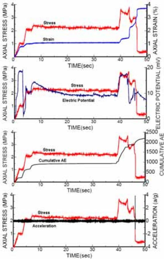
Figure 8 Multi-parameter response of Derinkuyu tuff
