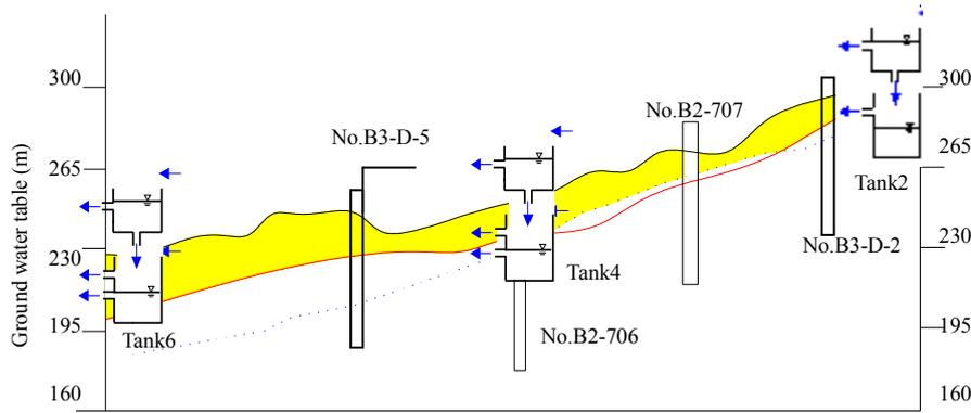
Fig.2 Configuration of multi-tank model in the slope
