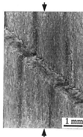
Fig. 5. Kink band in wood specimen. Axial stress direction is indicated by arrow.
