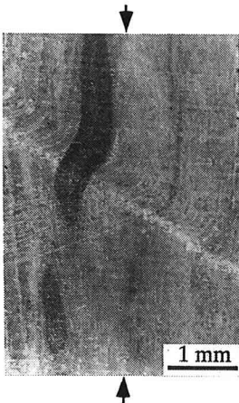
Fig. 4. Nucleation of kink showing folding into a very gentle monoclinal buckle. Axial stress direction is indicated by arrow.
