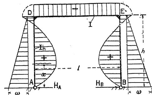
$$H_B = \frac{\left(1 + \frac{9}{10}\nu\right)}{12\left(1 + \frac{2}{3}\nu\right)} \cdot \omega \cdot h \quad \dots \dots \dots (1030)$$
