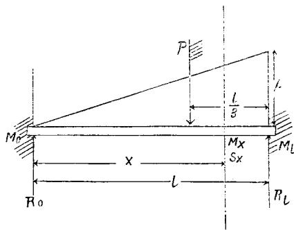
$$\text{From (13)} \quad M_x = -\frac{P l}{15} + \frac{3Px}{10} - \frac{Px^3}{3l^2} \quad \dots \dots \dots \quad (30)$$
