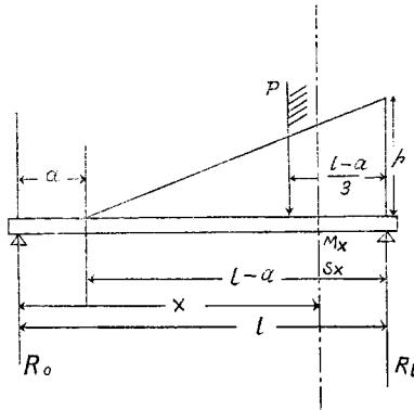
Since the beam under consideration is supported at both ends, the equations of bending moment at any point may be represented in the following forms:
