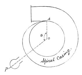
Let  $\theta$  = angle AOP measured from the beginning of the casing A. S' = sectional area of the spiral casing cut by a radial plane OP.
