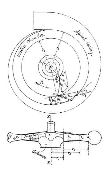
Let  $w_1$  and  $w_2$  be the absolute velocities of the fluid at the inlet and outlet surfaces of the impeller respectively.
