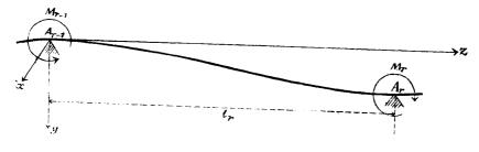
Let M denote the bending moment for rth span considered as a simple beam, then the reactions at  $A_{r-1}$  and  $A_r$  are
