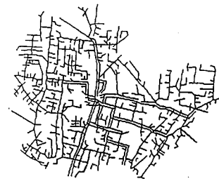
Fig.2 Electric powerline network (Minami Koizumi).
