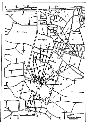
Fig. 4 Permanent ground displacement of the Southern part of Noshiro city during the 1983 Nihonkai-Chubu earthquake (after Hamada et al. , 1986).
