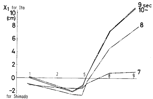
Fig. 5 Longitudinal Displacement due to Sub Fault in Infinite Medium
