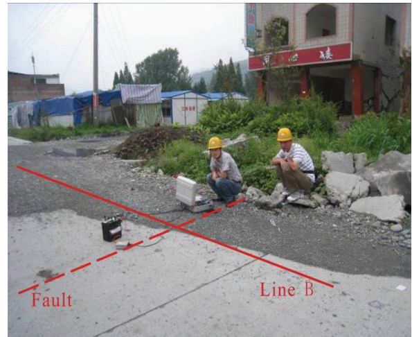
Figure9-2. Measuring points at the fault zone in the Xiaoyudong Town.
