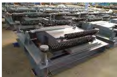
写真-1 5 Tuned Mass Damper
