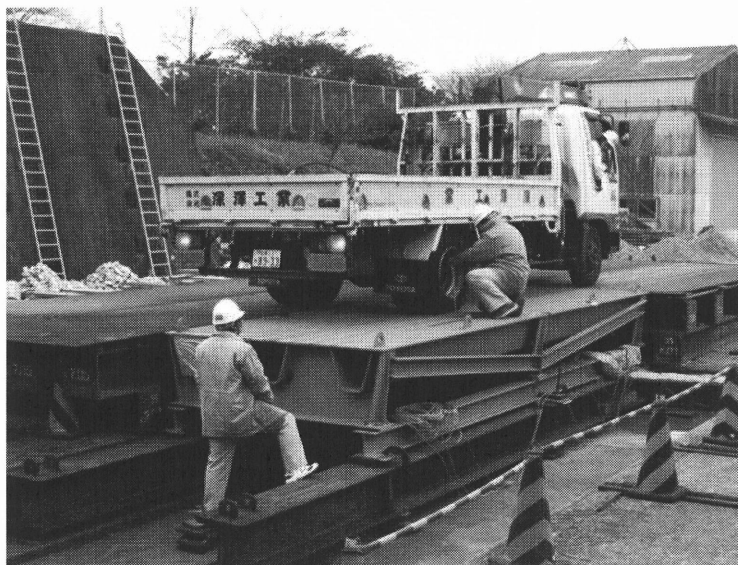
Fig. 13 Loading Test of Orthotropic Steel Deck
